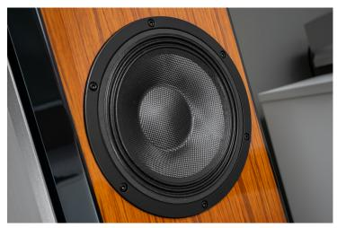
The multi-pleated surround of the woofer surrounds the cone and its shape ensures defined guidance: It combines the best possible freedom of movement for the vibrating surface and - in conjunction with the centring spider - ensures a controlled return of the cone to its rest position. In order to avoid unwanted vibrations and resonances, this special surround is provided with a damping coating.
