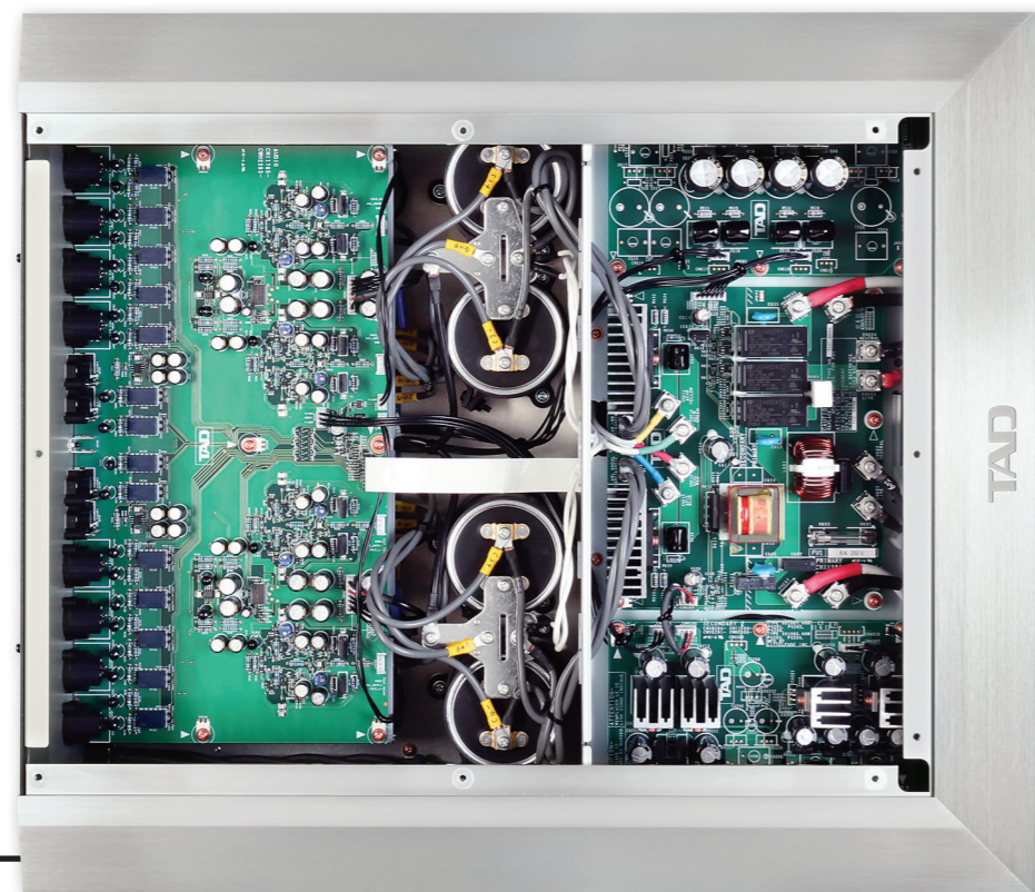
RIGHT: Single-stage current-feedback preamp [left] is fed from a separately regulated supply off the main twin-transformer/4x33,000µF PSU [right and centre]. The Class D output stage is under the top input switching/preamp PCB
