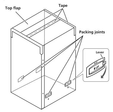
2. Using a screwdriver, remove the bolts and washers (six in all) from the packaging and open and remove the outer carton.
