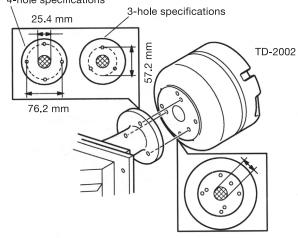
Use the accessory hexagonal screws  $(M6\times20)$  and flat washers, making sure that each is secured firmly. Note that incorrect horn mounting may well result in deterioration of the frequency response, and the generation of distortion. For a horn flange of less than 4 mm (5/32 in.) in thickness, the screws furnished with the unit cannot be used; use commercially
